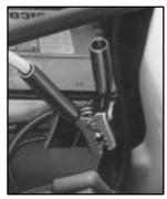
8. Now connect the black negative (-) cable to the good battery's negative (-) terminal.
